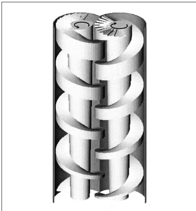
Figure 7. Twin screw extruder: extruder assembly.
